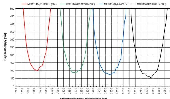
Fig. 12. Values of acceptable parameters of disturbances for new-type current jointless track circuit receivers
