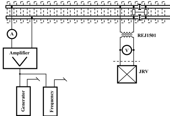
Fig. 4. Measurement system for field analysis of classic track circuit
